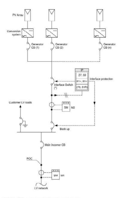
(\*) Motorized CB operated by undervoltage release or Contactor
