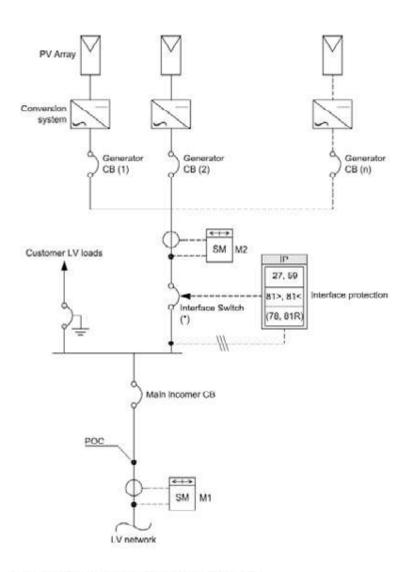
(\*) Motorized CB operated by undervoltage release or Contactor
