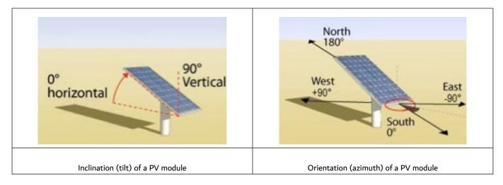
Figure 1 – Orientation and inclination of the PV panels
