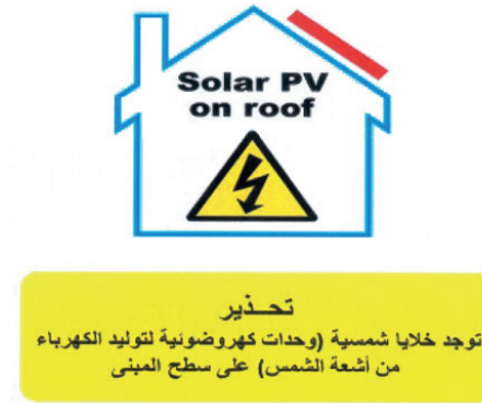
Figure 8 – Sign to be used to indicate the presence of a PV plant
