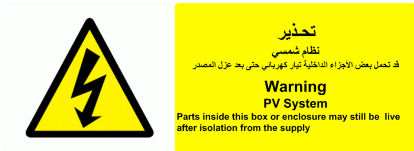
Figure 16 - Example of sign required on PV array combiner boxes (On-Site Guide BS 7671:2008 (2011))
