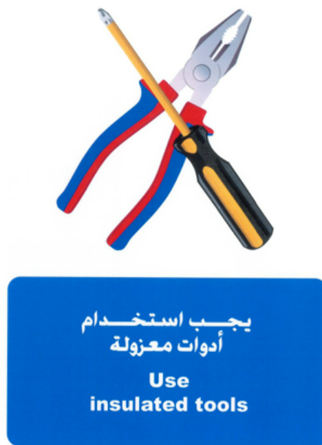
Figure 14 – Example of simplified layout indicating the compulsory use of insulated tools
