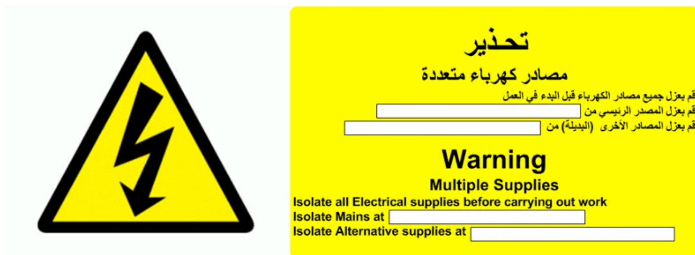
Figure 17 - Example of switchboard sign for identification of multiple supplies (On-Site Guide BS 7671:2008 (2011))
