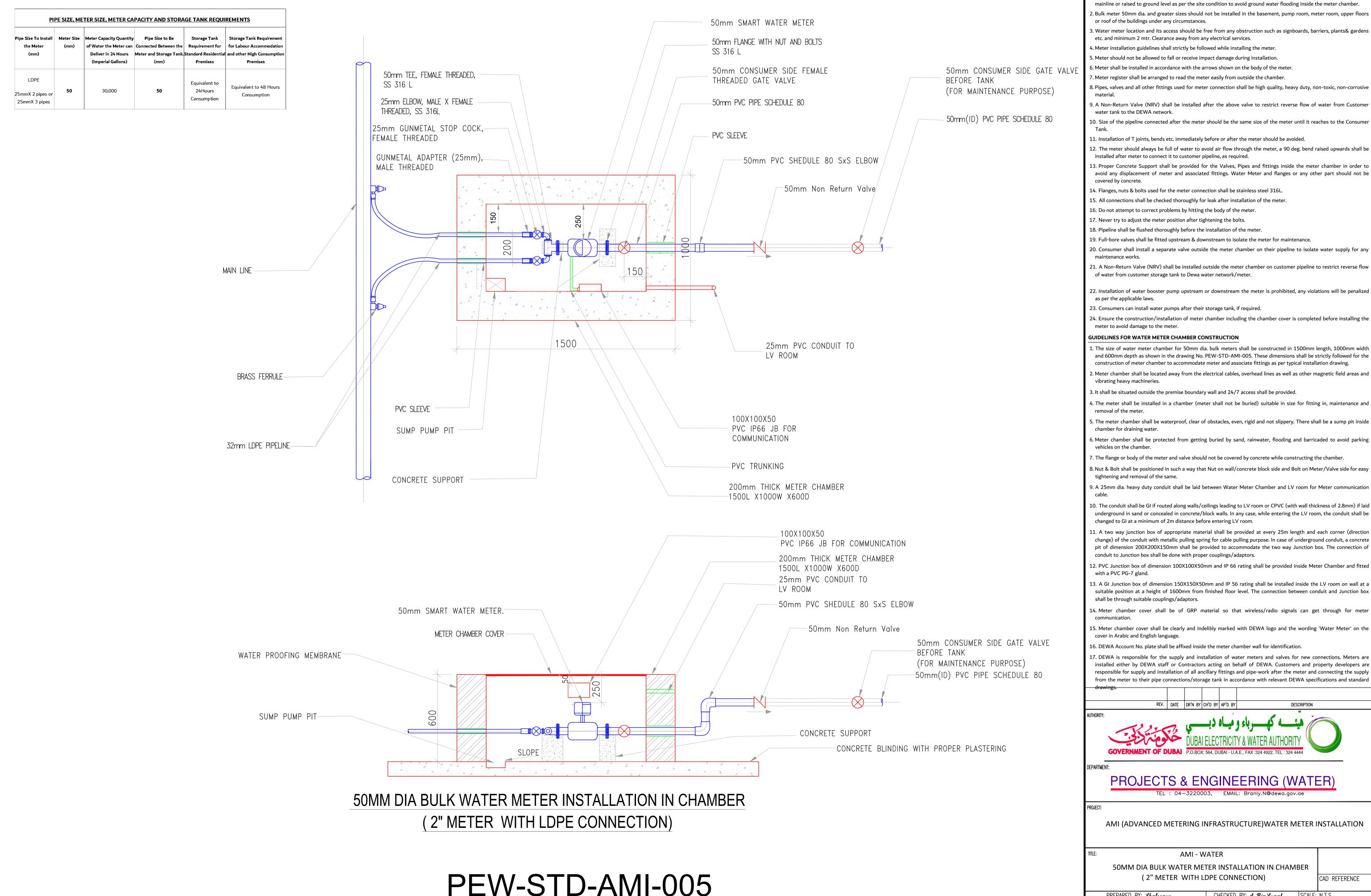
I. Water meters, 50mm dia. size shall be installed horizontally inside the meter chambers as shown in standard installatior drawing PEW-STD-AMI-005. These meters shall be installed in concrete waterproof chambers in the same level of
