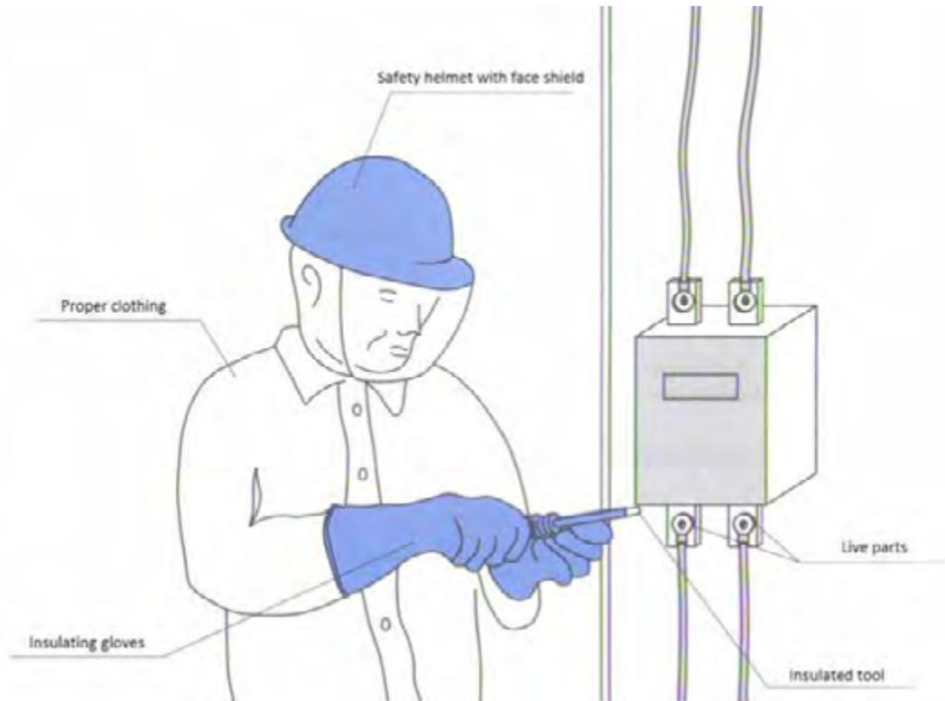
Figure 3 – Safety measures for works under voltage
