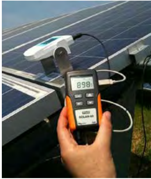
Figure 8 – Measurement of the solar irradiance from a reference solar cell. Example of a solar cell oriented as PV modules
